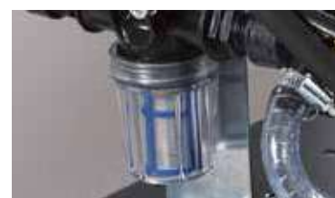
Readily serviceable external suction filter
