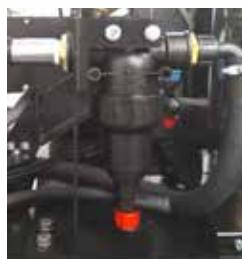
Direct water pumping system with self-cleaning filter and antiscale pump
